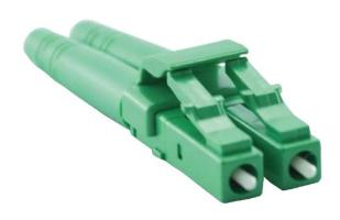
The LC connector features a 1.25mm Zirconia ferrule in a small form factor (SFF) fibre optic connector housing with a snag free latch which gives an audible click upon engaging for reliable and high density connections.
