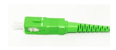
The SC connector features a 2.5mm Zirconia Ceramic ferrule and a push/pull coupling mechanism for a fast and reliable connection. A range of pigtail, Simplex and Duplex SC connectors are manufactured including Standard, Premium Low Loss and High Performance Grades which are suitable for various applications.
